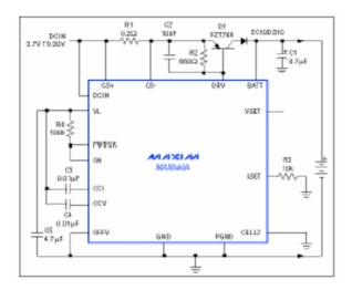
**Figure 1.** Designed for single lithium-ion cells, this battery-charging circuit is ideal for use in a stand-alone cradle charger.
