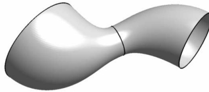
Figure 4: Two envelopes of 1-parameter families of spheres, joining smoothly.
