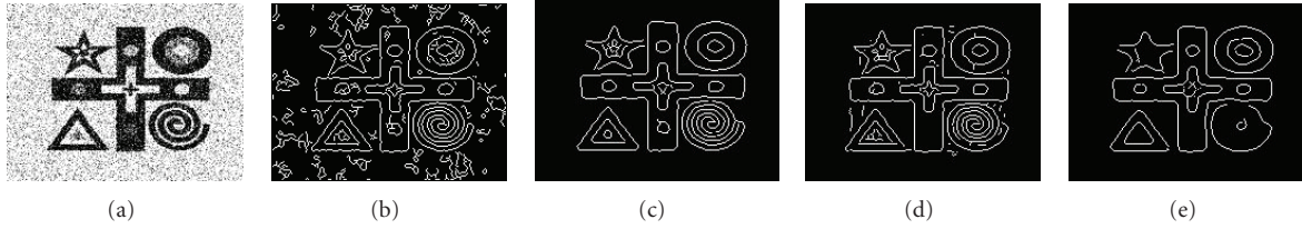
FIGURE 3: (a) A noisy image. (b) Its edge map given by Canny operator without any preprocessing. (c)–(e) are the edge maps of the given by Canny operator on the diffused images after applying the proposed method, TV, and the Perona-Malik methods, respectively.
