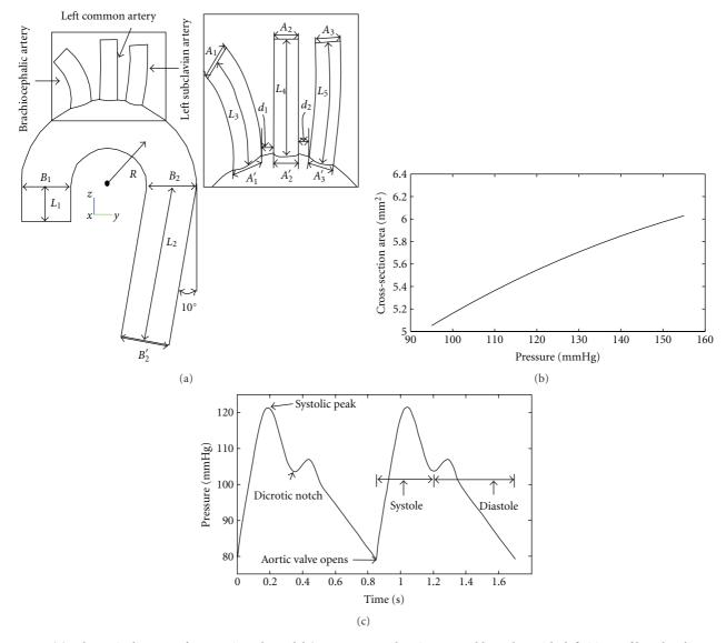
FIGURE 1: (a) Schematic diagram of 3D aortic arch model (Inset: a zoomed region around branches with definitions of lengths, diameters, and distances also common with the two other geometries), (b) the plot of luminal cross-sectional area of ascending aorta versus pressure estimated from Towfiq et al. [9]. (c) Pressure pulse at the inlet of ascending aorta under normal pressure condition.
