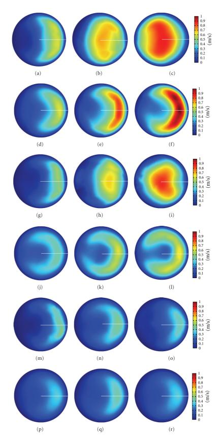
FIGURE 7: Axial velocity distributions at the axial cross-sections (a, b, c) D, (d, e, f) E, (g, h, i) F, (j, k, l) G, (m, n, o) H, (p, q, r) I (as shown in Figure 3(a)) through aortic arch at time t = 0.18 s, where a, d, g, j, m, and p correspond to hypotension; b, e, h, k, n, and q correspond to normal pressure; c, f, I, l, o and r correspond to hypertension.
