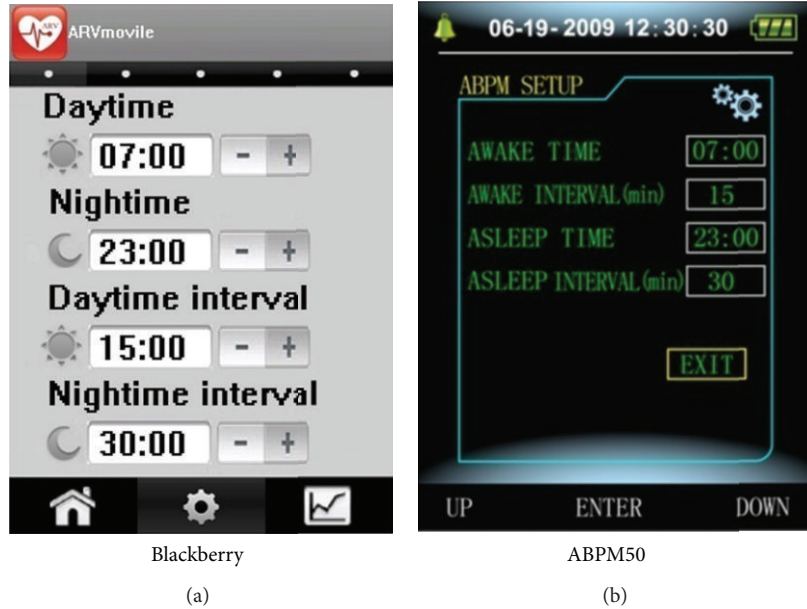
FIGURE 5: Matching daytime and nighttime thresholds and recording intervals on a Blackberry and ABPM50 graphic user interface.
