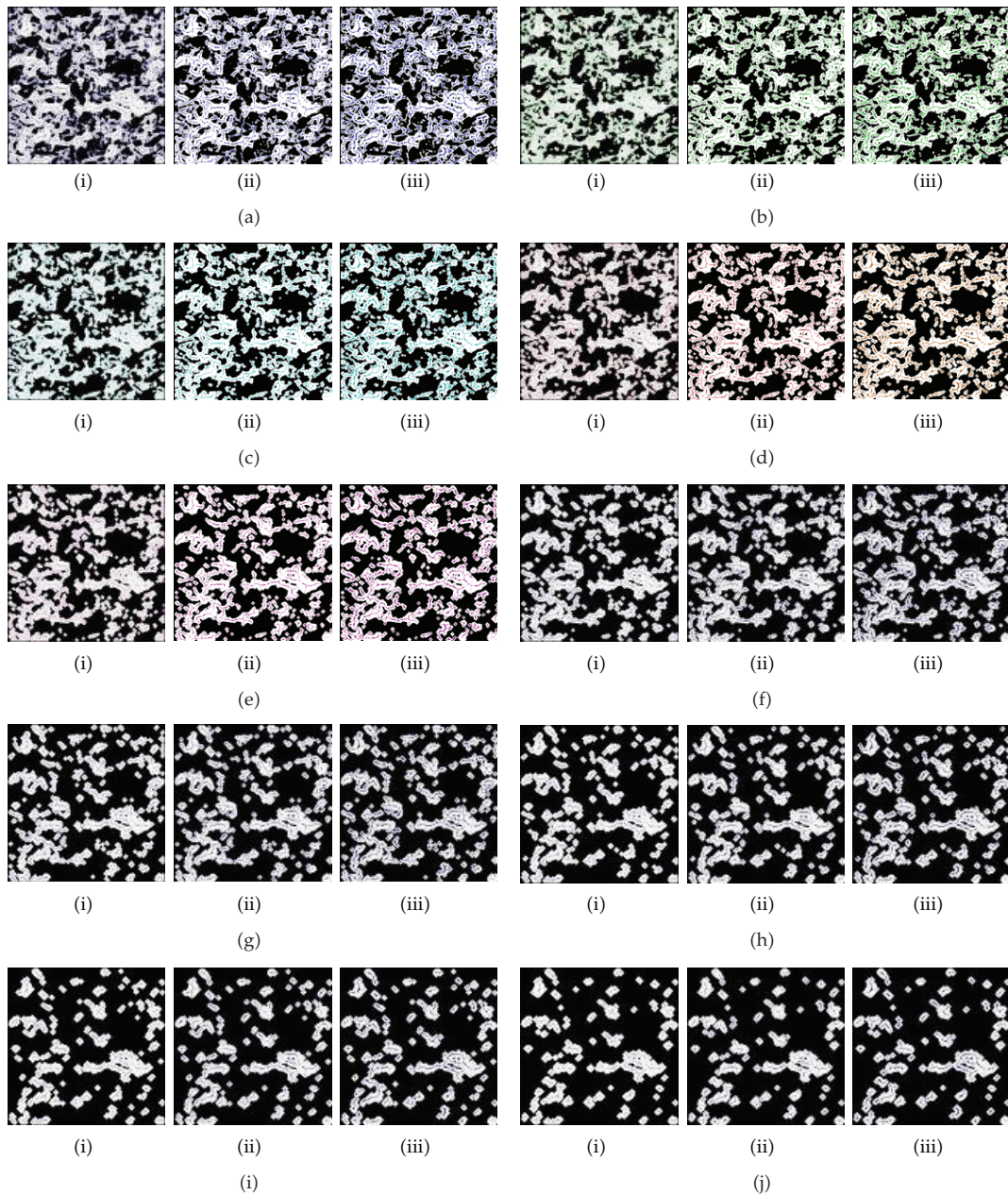
Figure 4: (a–j) The opening transformations of pore images in Figure 3(a)–3(j) are used to extract pore connectivity networks by structuring elements ((i) rhombus, (ii) square, and (iii) octagon).
