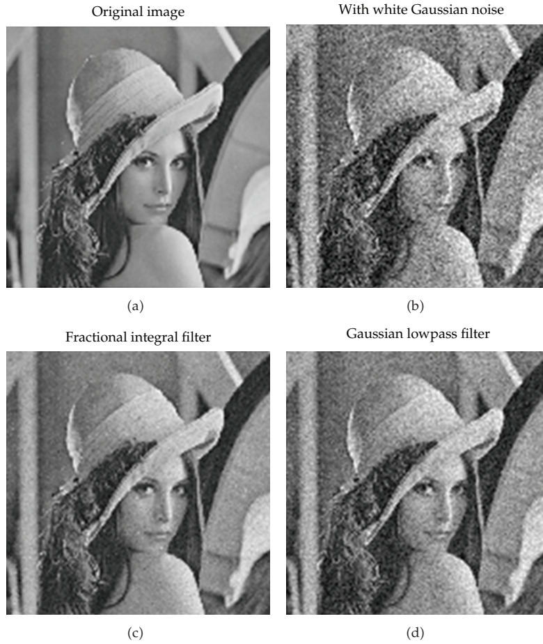
Figure 2: Results of denoising by fractional integral and Gaussian smoothing filter with noise variance = 0.01.
