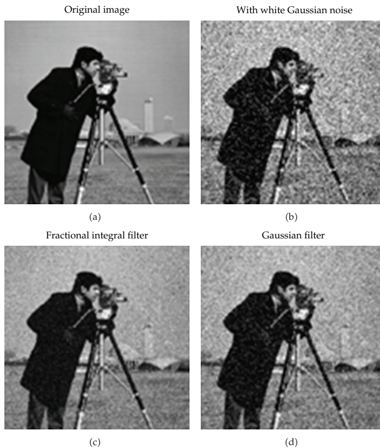
Figure 3: Results of denoising by fractional integral and Gaussian smoothing filter with noise variance = 0.02.
