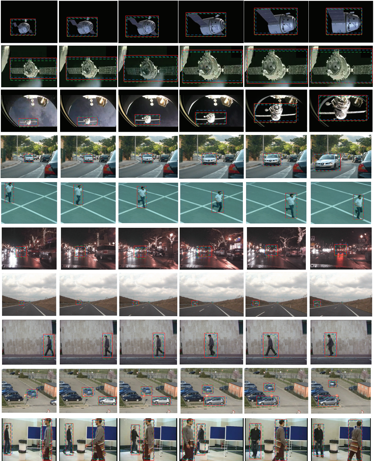
FIGURE 4: Experimental results from the tracking, marked by the bounding box. The red (solid line) box is from our proposed method, the blue (dashed line) box is Tracker-1 from the particle filters in [27], and the green (dashed line) box is Tracker-2 from the online distance metric learning in [28]. The rows 1–10 contain images from the videos “Satellite-1,” “Satellite-2,” “Satellite-3,” “Automobile-1,” “Running,” “Automobile-2,” “Highway,” “Walking,” “Automobile-3” and “Walking-2,” respectively.
