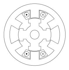
Figure 2.1. A 3-phase, 6/4 VRM. One-phase winding is shown.
