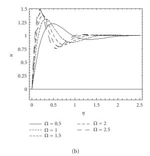
Figure 4.1. Effect of  $\Omega$  on real part of velocity profile *u* versus  $\eta$ . In (a) for Newtonian fluid at  $\alpha = 0$ ,  $\omega t = \pi/2$ , A = 0.2,  $\epsilon = \omega = 0.5$ ,  $W_0 = -0.5$ ,  $\nu = 0.1$ . In (b) for second-grade fluid at  $\alpha = 0.4$ .
