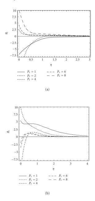
Figure 4.6. Effect of  $P_r$  on imaginary part of temperature profile  $\theta_i$  versus  $\eta$ . In (a) for Newtonian fluid at  $\alpha = 0$ ,  $\omega t = \pi/2$ ,  $A = \epsilon = \omega = 0.5$ ,  $W_0 = -0.5$ ,  $\nu = 0.1$ ,  $\Omega = 2.5$ ,  $E_c = 5.0$ , k = 0.2, P = 0.3. In (b) for second-grade fluid at  $\alpha = 0.04$ .
