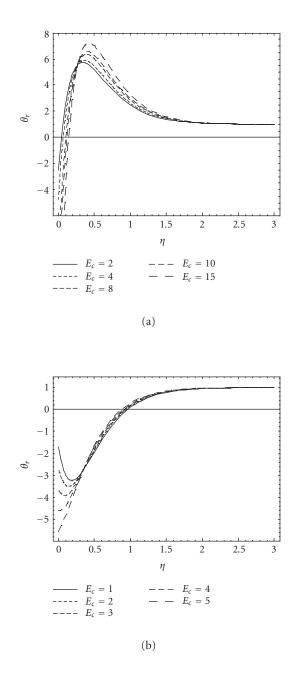
Figure 4.7. Effect of  $E_c$  on real part of temperature profile  $\theta_r$  versus  $\eta$ . In (a) for Newtonian fluid at  $\alpha = 0$ ,  $\omega t = \pi/2$ ,  $A = \epsilon = \omega = 0.5$ ,  $W_0 = -0.5$ ,  $\nu = 0.1$ ,  $\Omega = 4.0$ ,  $P_r = 5.0$ , k = 0.2, P = 0.3. In (b) for second-grade fluid at  $\alpha = 0.04$ .
