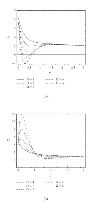
Figure 4.3. Effect of  $\Omega$  on real part of temperature profile  $\theta_r$  versus  $\eta$ . In (a) for Newtonian fluid at  $\alpha = 0$ ,  $\omega t = \pi/2$ ,  $A = \epsilon = \omega = 0.5$ ,  $W_0 = -0.5$ ,  $\nu = 0.1$ ,  $P_r = 1.5$ ,  $E_c = 5.0$ , k = 0.2, P = 0.3. In (b) for second-grade fluid at  $\alpha = 0.04$ .
