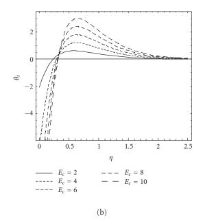
Figure 4.8. Effect of  $E_c$  on imaginary part of temperature profile  $\theta_i$  versus  $\eta$ . In (a) for Newtonian fluid at  $\alpha = 0$ ,  $\omega t = \pi/2$ ,  $A = \epsilon = \omega = 0.5$ ,  $W_0 = -0.5$ ,  $\nu = 0.1$ ,  $\Omega = 2.5$ ,  $P_r = 5.0$ , k = 0.2, P = 0.3. In (b) for second-grade fluid at  $\alpha = 0.05$ .
