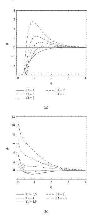
Figure 4.4. Effect of  $\Omega$  on imaginary part of temperature profile  $\theta_i$  versus  $\eta$ . In (a) for Newtonian fluid at  $\alpha = 0$ ,  $\omega t = \pi/2$ ,  $A = \epsilon = \omega = 0.5$ ,  $W_0 = -0.5$ ,  $\nu = 0.1$ ,  $P_r = 1.5$ ,  $E_c = 5.0$ , k = 0.2, P = 0.3. In (b) for second-grade fluid at  $\alpha = 0.05$ .
