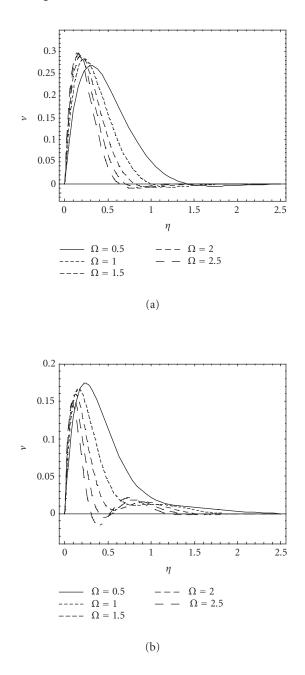
Figure 4.2. Effect of  $\Omega$  on imaginary part of velocity profile  $\nu$  versus  $\eta$ . In (a) for Newtonian fluid at  $\alpha = 0$ ,  $\omega t = \pi/2$ , A = 0.2,  $\epsilon = \omega = 0.5$ ,  $W_0 = -0.5$ ,  $\nu = 0.1$ . In (b) for second-grade fluid at  $\alpha = 0.1$ .
