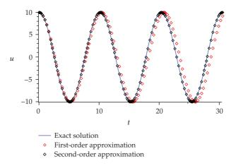
**Figure 5:** Comparison of approximate periodic solutions of Bucking of a Column equation (Case 1) with the exact one for  $m = l = P = k_1 = 10.0$ , and  $k_3 = 50.0$  with u(0) = 10.0.
