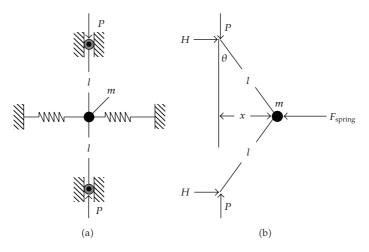
Figure 1: Model for the bulking of a column [2].
