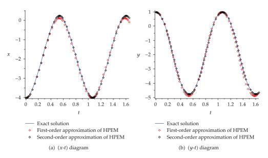
**Figure 9:** Comparison of the first- and second-order analytical approximate solutions with the exact solution for  $m_1 = 1.0$ ,  $m_2 = 2.0$ ,  $k_1 = 5.0$ ,  $k_2 = 1.0$  with x(0) = -4.0 and y(0) = 1.0 (Case 3).
