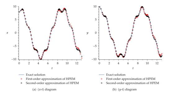
**Figure 8:** Comparison of the first- and second-order analytical approximate solutions with the exact solution for m = 2.0,  $k_1 = 1.0$ ,  $k_2 = 3.0$ ,  $k_3 = 5.0$  with x(0) = 8.0 and y(0) = 10.0 (Case 2).
