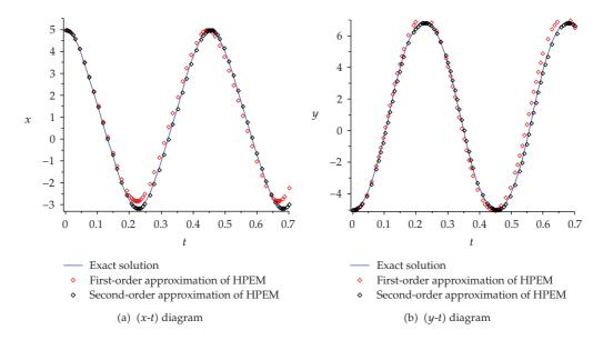
**Figure 10:** Comparison of the first- and second-order analytical approximate solutions with the exact solution for  $m_1 = 3.0$ ,  $m_2 = 5.0$ ,  $k_1 = 2.0$ ,  $k_2 = 5.0$  with x(0) = 5.0 and y(0) = -5.0 (Case 3).
