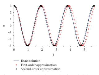
**Figure 4:** Comparison of approximate periodic solutions of Bucking of a Column equation (Case 1) with the exact one for m = 1.0, l = 1.5, P = 5.0,  $k_1 = 5.0$ , and  $k_3 = 6.0$  with u(0) = 3.0.
