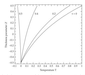
**Figure 1:** Through-the-thickness variation of dimensionless temperature T of FGM square plate for different values of the time parameter t.
