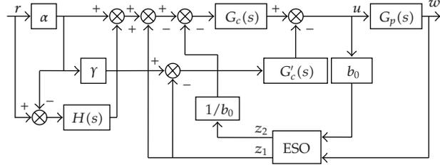
Figure 2: 2DOF Control Configuration Base on ESO.
