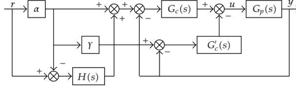
Figure 1: 2DOF Control Configuration.
