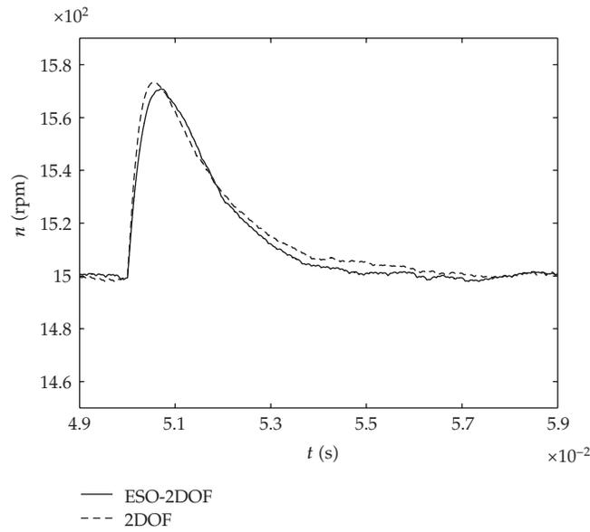
Figure 6: Dynamic speed response curves of PMSM system with unloading.
