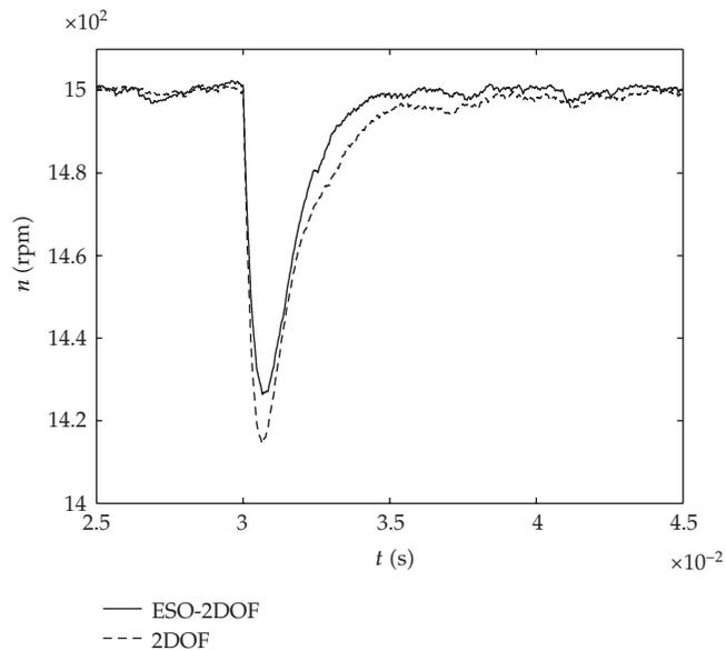
Figure 5: Dynamic speed response curves of PMSM system with parameter perturbation.
