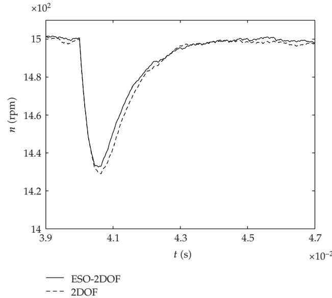
**Figure 3:** Dynamic antidisturbance curves of PMSM system.
