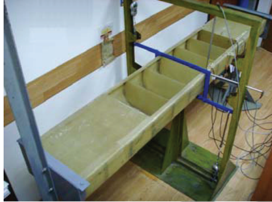
Figure 10: Ship hull model and torsion rig.
