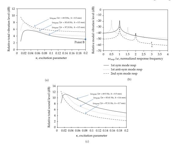
**Figure 4:** (a) Relative total vibration level  $(\omega_{\text{sym}}/\omega_{\text{anti-sym}} = 1.85, \omega = \omega_{\text{sym}})$ , (b) relative modal vibration levels of point B in (a), (c) relative total sound level  $(\omega_{\text{sym}}/\omega_{\text{anti}} = 1.85, \omega = \omega_{\text{sym}})$ .
