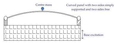
Figure 1: Side view of a curved panel mounted with a mass.
