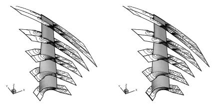
Fig. 5. (a) Rotor, TVD MacCormack scheme, (b) Rotor, Ni's scheme
