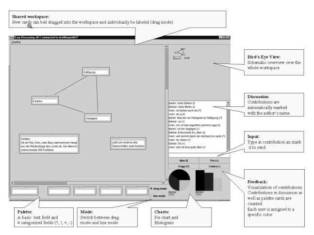
Figure 2. The design of the communication platform EasyDiscussing
